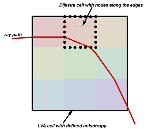
**Figure 3.** Each LVA cell has a single defined anisotropy, and is split into multiple Dijkstra cells with edges joining nodes on the cell sides. The shortest path follows these edges, and can bend within the LVA cell.
